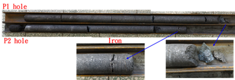
Fig.8. Samples taken from the core drilling of P1 hole and P2 hole
