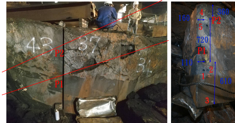
Fig.9. Investigation of the salamander tapping paths at No.3 BF
